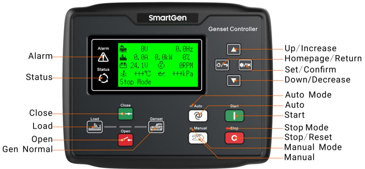
Fig.1 – HGM6110 (HGM6110N/NC/CAN) Front Panel Indication
