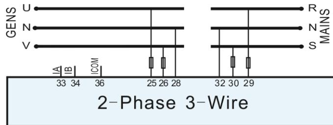
Fig.9 - 2-Phase 3-Wire Connection Diagram
